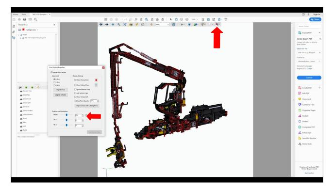
And you can also make section views (top arrow) and by moving this slider (arrow below left) you can slice through the model where you want it in the x, y, or z direction. Here it is the Y-Axis, see in the window.
