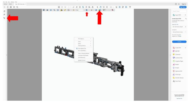
Show Model Tree. There are possibilities to open more Toolbars where you also can toggle the Model Tree: in the window above, click *Tools* and then at the bottom of the next window *Open Toolbar*.
