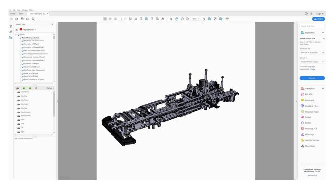
Here you see sub-assemblies and parts together in the REN-106-Frame Assembly. The subassemblies you have build before, so you don't have to see their parts now. To prevent the computer from getting slow, there are a great number of parts removed from the sub-assemblies before placing them here and you see the text *Outlines* behind the name now.
