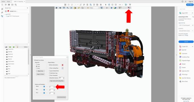
And you can also make section views (top arrow) and by moving this slider (arrow below) you can slice through the model where you want it.
