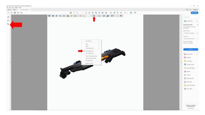
Click here to open the Model Tree. The Model Tree shows a list of all parts and sub-assemblies in the building sequence.
