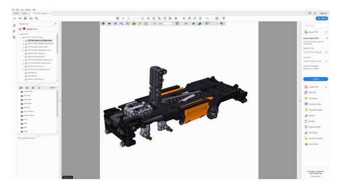
Here you see sub-assemblies and parts together in the CRT-107-Frame Assembly. The sub-assemblies you have build before, so you don't have to see their parts now. To prevent the computer from getting slow, there are a great number of parts removed from the sub-assemblies before placing them here and you see the text *Outlines* behind the name now.
